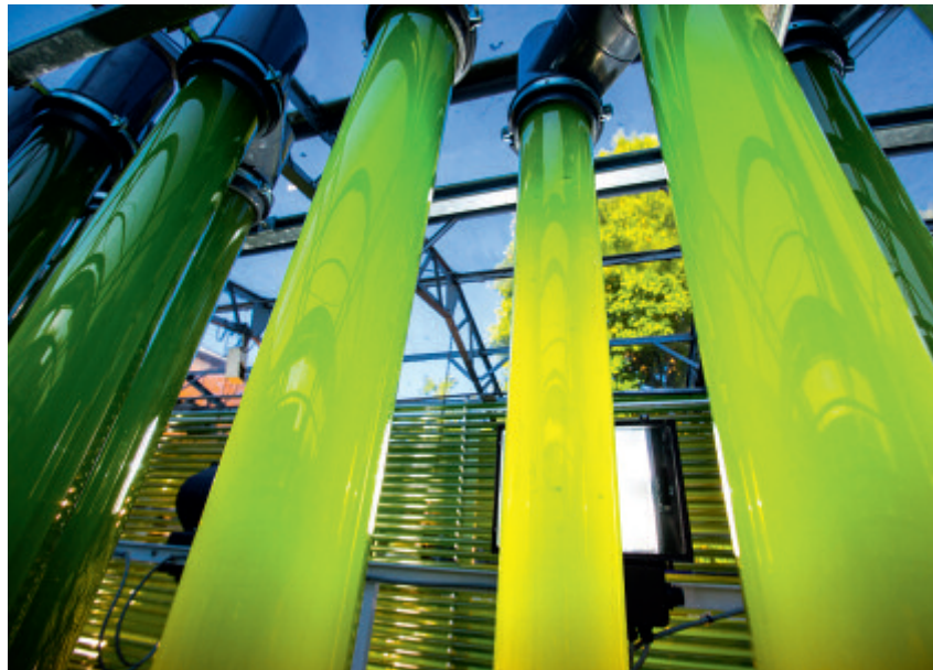
Closed photo bioreactor for cultivating microalgae at Swansea University (project EnAlgae)
