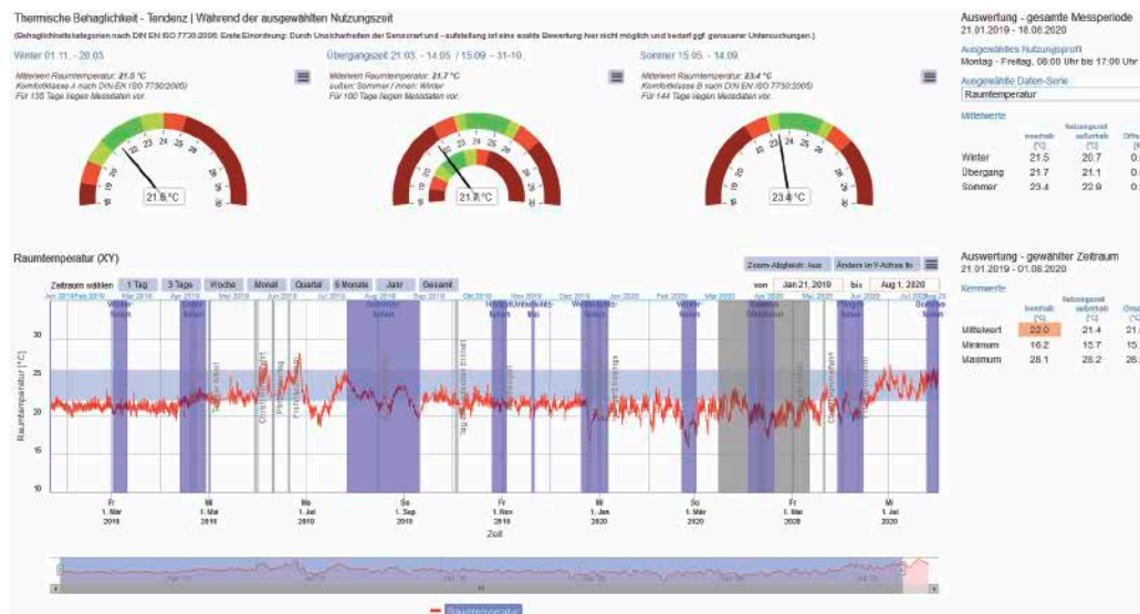
Figure 100: Evaluation of the air temperature in a common room within the extension at Giebelstadt Primary School for the period between January 2019 and July 2020, on the online platform provided by Dresden University of Technology Source: Dresden University of Technology
