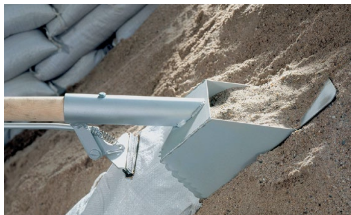
A simple tool for filling sandbags
