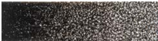
Reticulated polyurethane foam, source: ILEK
