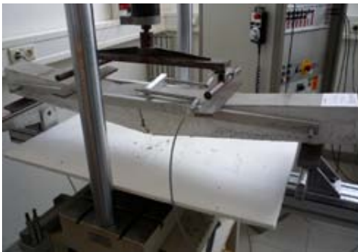
4-point bending-tensile trial, source: ILEK
