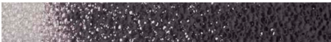
Graduated infiltration of reticulated polyurethane foam with glue cement in the interest of varying stiffness, source: ILEK
