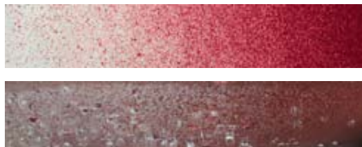
Top: glass fibre texture with silicon elements for graduated permeability
