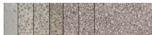
Top: testing varying-density aerated concrete Bottom: homogenous concrete mixtures in levels of graduated density for material testing [2], source: ILEK
